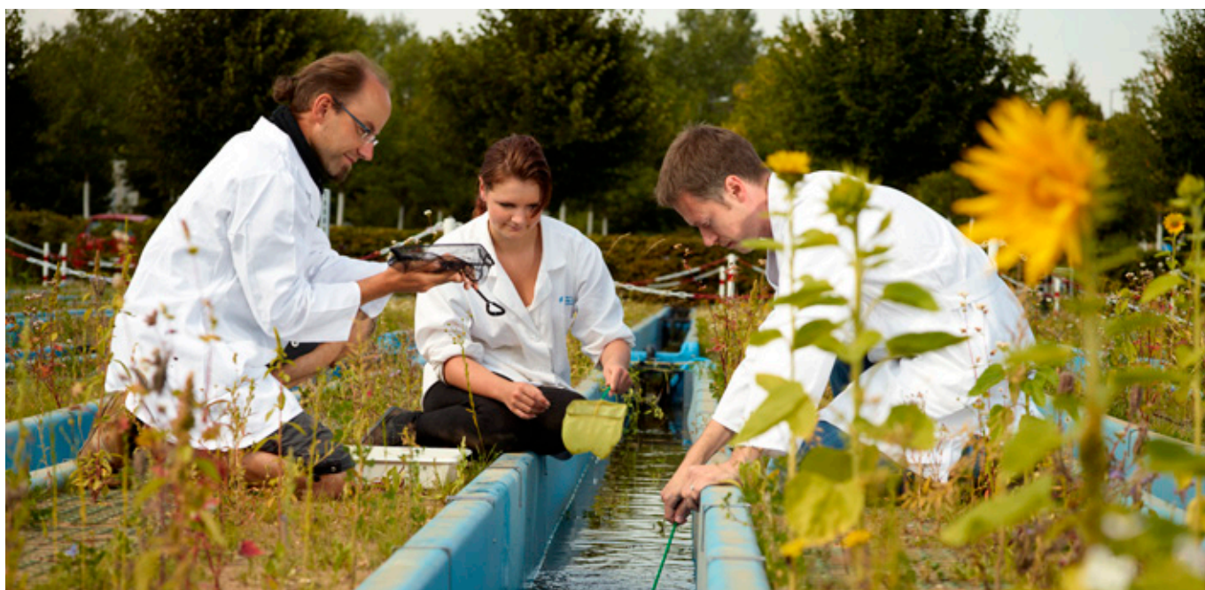
The UFZ's river experiment with 47 fourteen-meter long artificial gutters helps to investigate the effects of pesticides on aquatic organisms under considerably more realistic conditions than in the laboratory.
